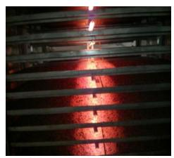
Fig. 2 Neem fruit at drying chamber in an infrared cabinet dryer
