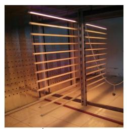
Fig. 3 Infrared Cabinet Dryer
