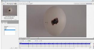
Figure 3. Primary dirtiness measurement process by using LabVIEW Vision Assistant software
