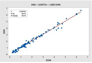
Figure 9. LabVIEW Vision Assistant – Image and Video measurement regression value and estimation equation which belongs to dirty white egg samples
