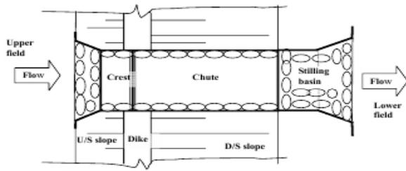
Figure 1 Schematic layout plan of a terrace structure
