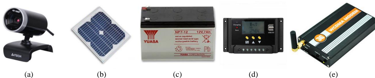
Figure 1 a) HD camera, b) solar cell, c) 12v 7Ah battery, d) charging unit, e) 3G GPRS modem
