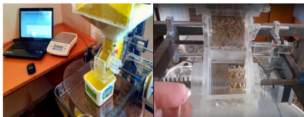
Figure 1. General (left) and close view (right) of the test unit equipped with fluted rolls as manufactured to determine the volumetric efficiency
