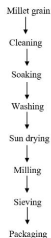
Figure 2ç Flow chart for the production of millet flour (Egwujeh et al., 2016a)
