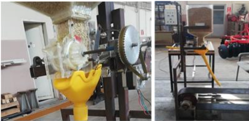
Figure 2. Closed view of metering unit with fluted roll (left) and setup on sticky belt test stand (Right)
