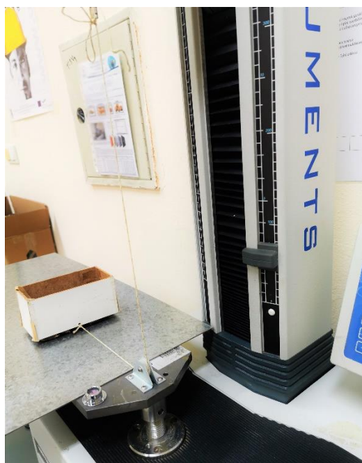
Figure 3. Wooden box used in friction tests
