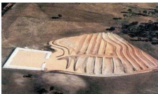
Figure 6. Row spacing system collecting surface runoff in a pond in Australia (Incebel, 2012).
