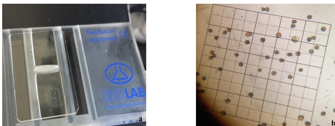
Figure 2. Visuals of hemocytometric microscope slide (a) and the pollens that appear on the ocular micrometer (b)
