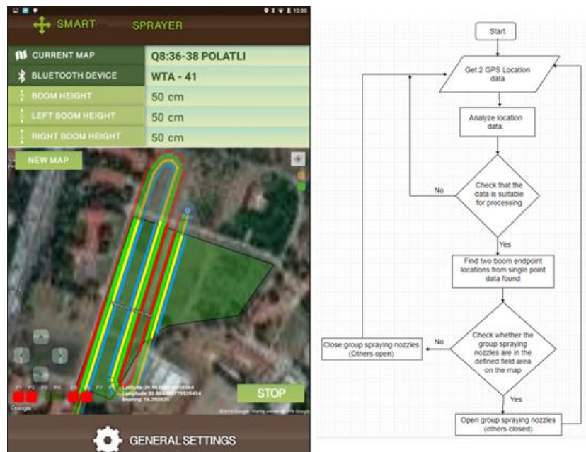
Figure 5. Interface and flow diagram of the state of active operation and group-operated solenoid valves.
