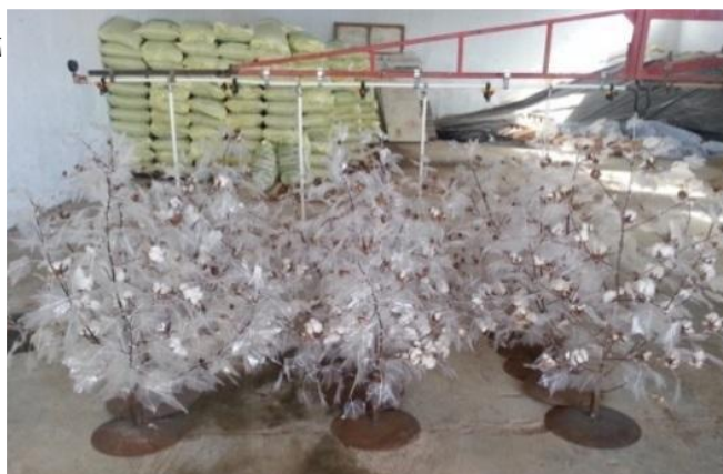
Figure 1. The image of the spray nozzle positions using the upper and under leaves
