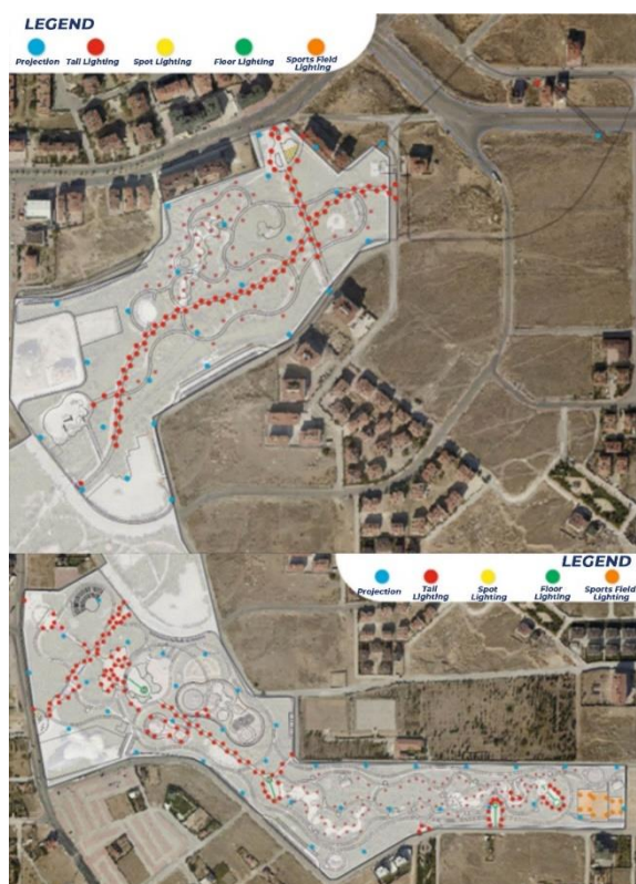
Figure 3. Locations of Existing Lighting Elements in Butterfly Valley Park
