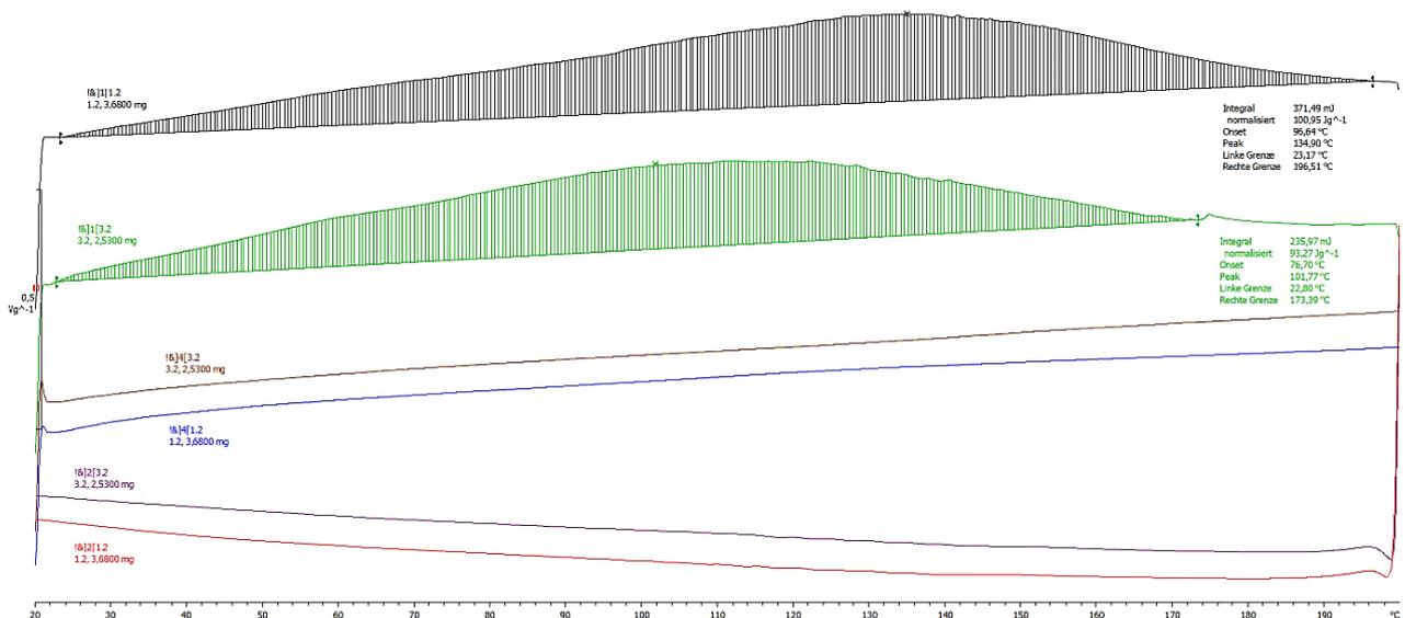
Figure 7. DSC graphs of the sol-gel coated biocomposite films
