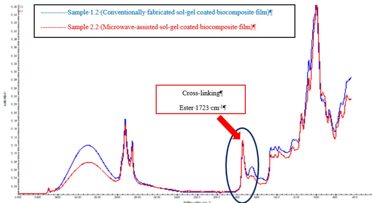
Figure 5. FT-IR spectra of the the sol-gel coated biocomposite films
