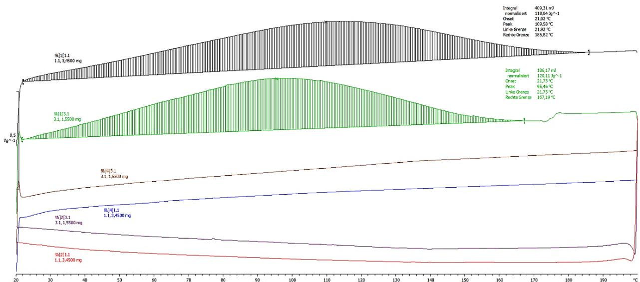
Figure 6. DSC graphs of the non-coated biocomposite films
