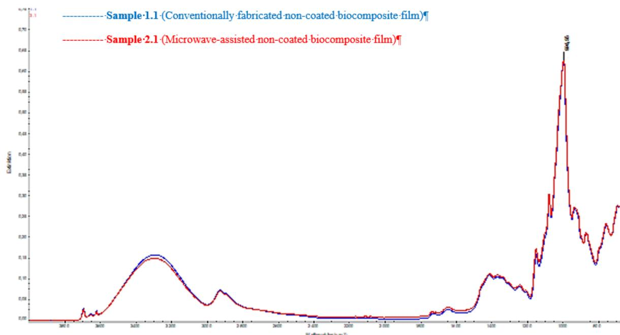
Figure 4. FT-IR spectra of the non-coated biocomposite films
