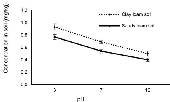
Figure 4 Effect of pH on adsorption
