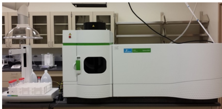
Figure 3. Coupled Plasma Optical Emission Spectroscopy (ICP-OES)
