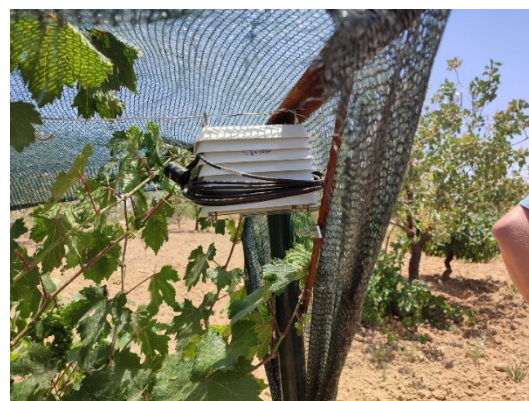
Figure 2. HOBO U12-013 installed in the vineyard
