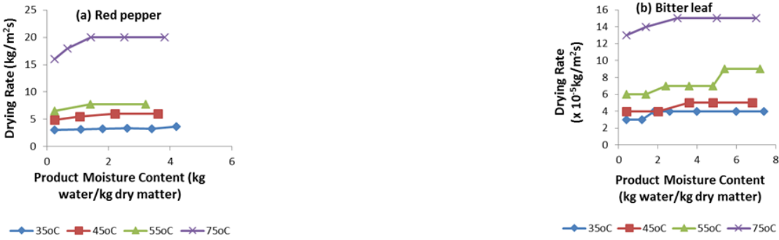
Figure 2 Variation of drying rates with product moisture content for (a) Red pepper (b) Bitter leaf
