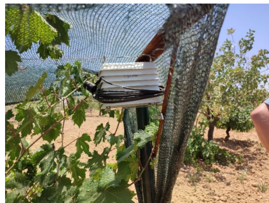
Figure 2. HOBO U12-013 installed in the vineyard
